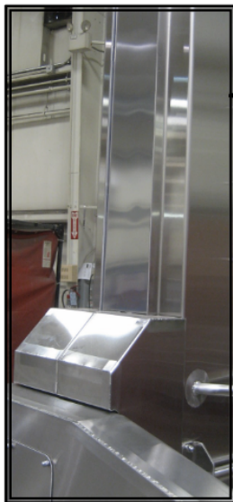
1. Stainless steel magnetically sealed slot cover
